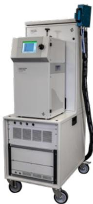
The model 3095 Engine Exhaust Particle Measurement System (EPPMS) is a turn-key emissions measurement solution that combines the 3090 EEPS™ and the 3098 Porous Tube Thermodiluter (PTT). The model 3098 consists of two porous tube diluters (hot first stage and room-temperature second stage) and a catalytic stripper to remove volatiles. The system is fully characterized for losses and is controlled from the EEPS™ software for a seamless user experience.
