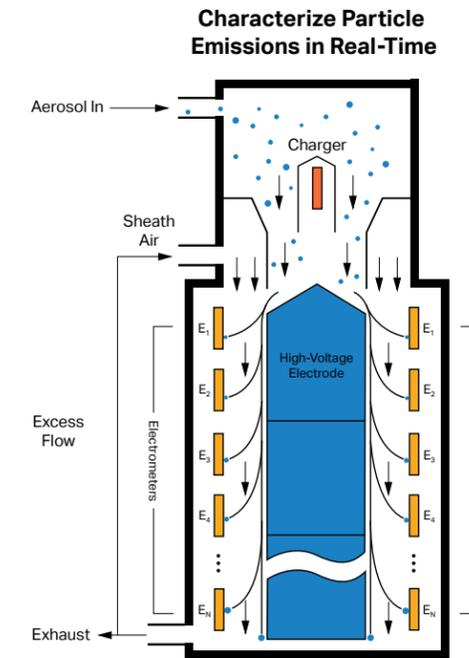
Figure 3. EEPS™ Flow Schematic
