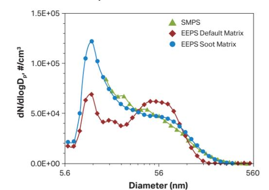
Figure 4. The number distribution of engine emissions as measured by an SMPS, and by the EEPS™ using two data inversion matrices.
