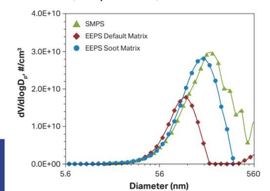
Figure 5. The volume distribution of engine emissions as measured by an SMPS, and by the EEPS™ using two data inversion matrices.
