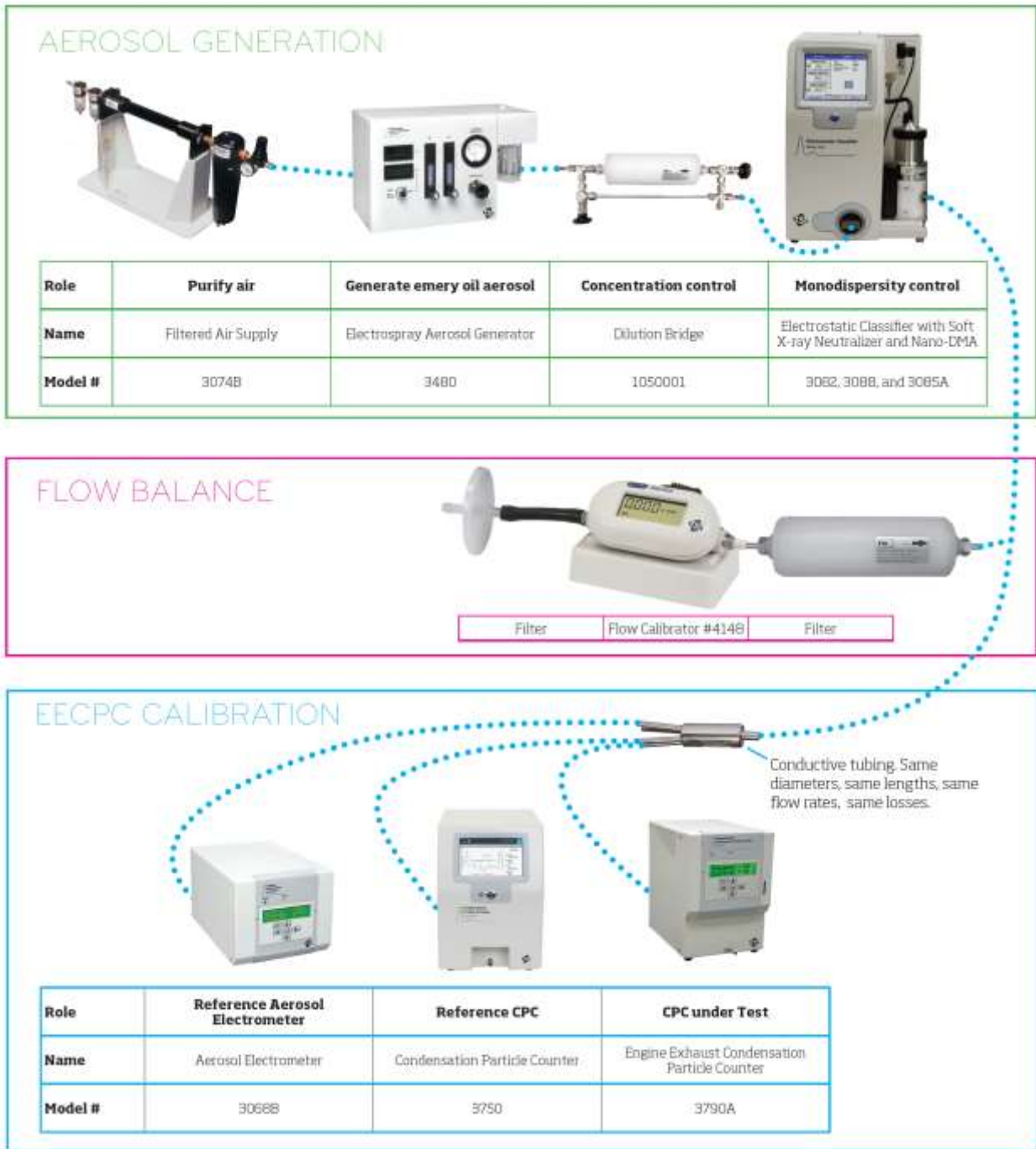
Figure 1: Schematic of the EECPC Calibration Setup
