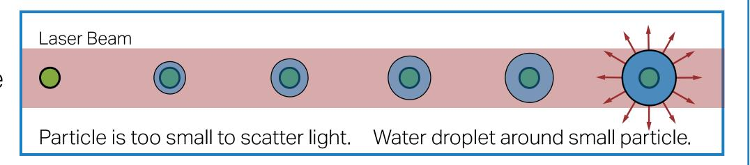
Why Water? Many other CPCs condense butanol or isopropyl alcohol onto the sampled particles. Compared to those materials, water is safe, eco-friendly, and easily available. Using water as a working fluid eliminates the potential for problems measuring high-humidity samples, which can occur when using an alcohol-based instrument. Since water and alcohol respond differently to different materials, the minimum detectable particle size may be slightly affected by particle composition.
