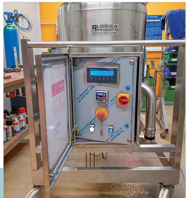
Weight indicator X3 for magnetic mixer control mounted on the front panel. The mobile mixer with weighing module Novego is made entirely of stainless steel, in order to ensure maximum sterility
