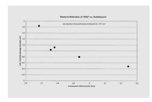
Table 18407 shows that the membrane material 18407 should not to be used as a sterile grade filter. This membrane only does have a retention rate of LRV 5.
