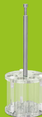
Basket type A (with 6 test tubes or type B with 3 test tubes)
