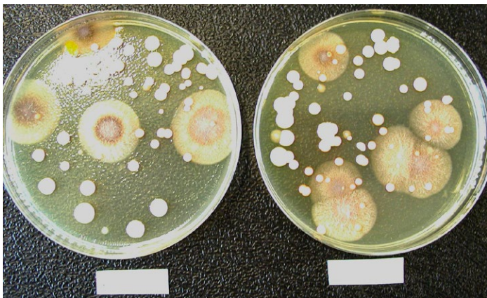
Figure 3: Comparison of the microbiological flora grown on a test filter (left) and its corresponding reference filter (right). The composition of the microbiological population found on the test and reference filters is comparable. Representative soybean-casein-digest agar medium plates showing the microbiological flora grown on a test filter (left) and its corresponding reference filter (right).
