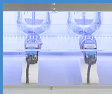
24/7 testing with LED light bar and six ethernet cameras.
