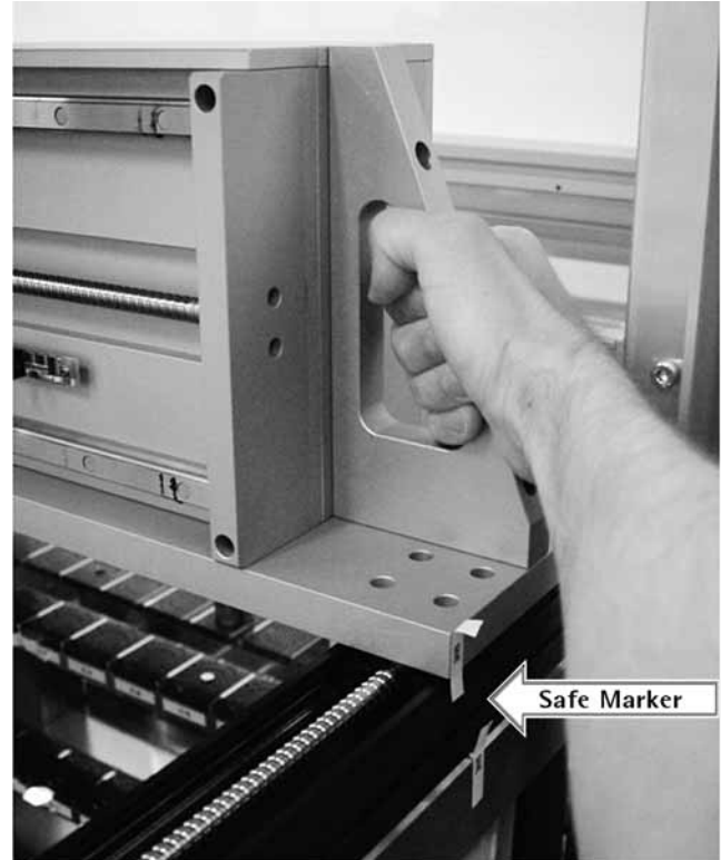
Figure 33: Holding point for sliding the portal into the safe corridor
