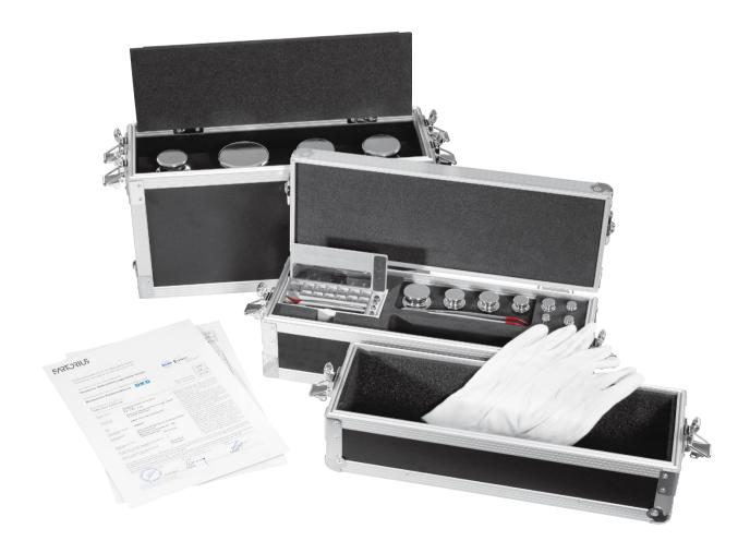
The Sartorius density reference set\* consists of stackable disc weights. All weights are made of special stainless steel that has a density of 8,000 kg/m<sup>3</sup>. Their tolerances comply with OIML R111-1. Density reference weights are non-magnetizable and are supplied in a high-quality wooden case with a calibration certificate, which includes density determination data.
