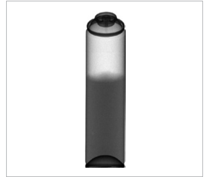
Fill level monitoring
