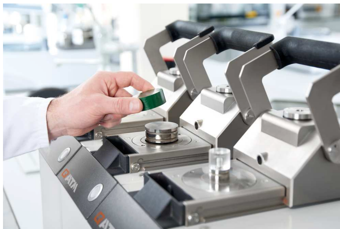
4. Start the mounting method with multifunctional button
