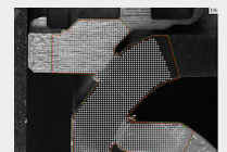
Test point pattern on a non-bedded specimen
