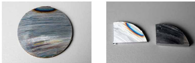
Figure 4. Samples which were cut with inappropriate cutting parameters
