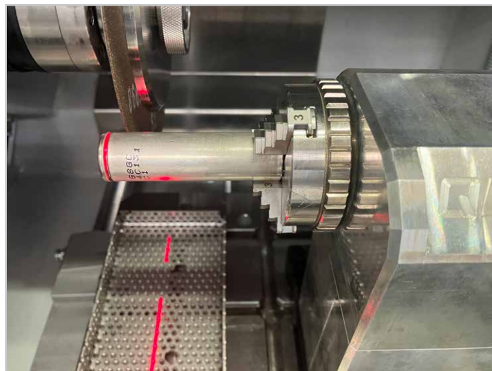
Figure 2: How to clamp the LIB in rotational clamping tool to cut the cap and take the jelly roll out.
