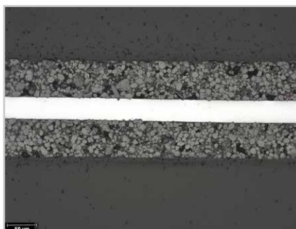
Figure 13: Aluminum foil coated on both sides with metal-oxide particles.
