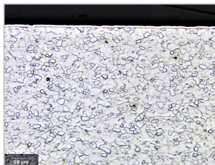
Figure 3 (left): The microstructure of the cap of a LIB after etching with 3% alcoholic nitric acid.
