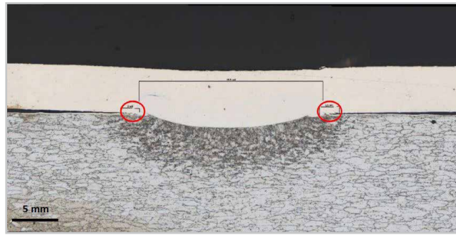
Figure 16: The spot welds on the cap of the battery. The red circles show tiny cracks on both ends of the spot weld. 3 % alcoholic nitric acid has been used as etchant [5].
