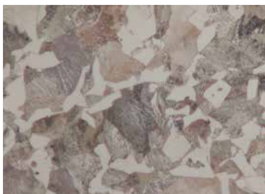
Figure 3: Ferrite-Pearlite, etched with 3% Nital, brightfield 20x
