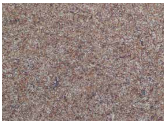
Figure 4: Martenitic structure after heat treatment, etched with 3% Nital, brightfield 20x
