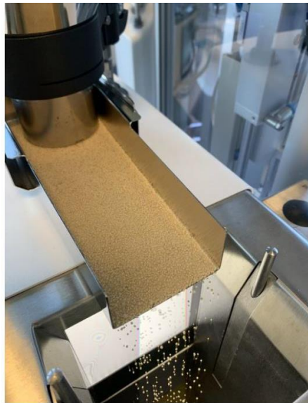
Fig.1: Limestone pellets during the measurement with the CAMSIZER 3D.
