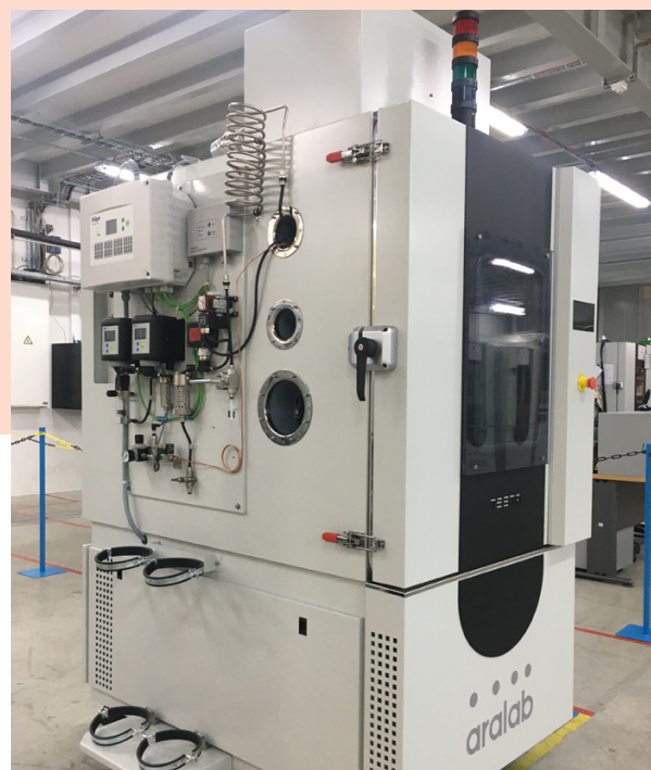
EUCAR Battery testing
