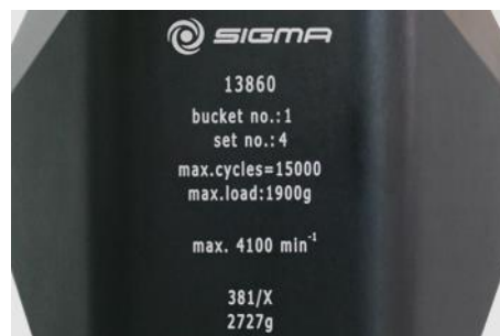
Fig. 5: Different service life – engraving on the bucket/rotor
