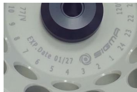
Fig. 5: Different service life – engraving on the bucket/rotor
