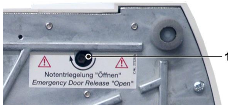
Fig. :15 Opening for the emergency lid release at the bottom of the centrifuge
