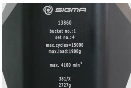
Fig. 2: Different service life – engraving on the bucket/rotor
