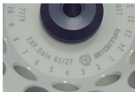
Fig. 2: Different service life – engraving on the bucket/rotor
