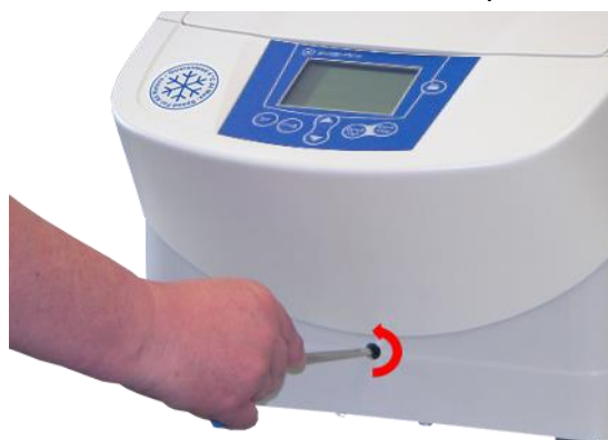
Fig. 15: Manual release of the lid lock
