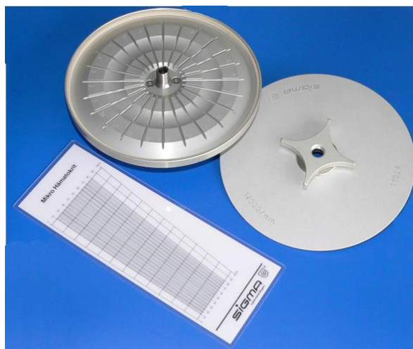
Fig. 7: Microhaematocrit rotor (part no. 11024) with reader (part no. 17029)
