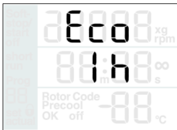
Fig. 12: Adjusting the turn-off time
