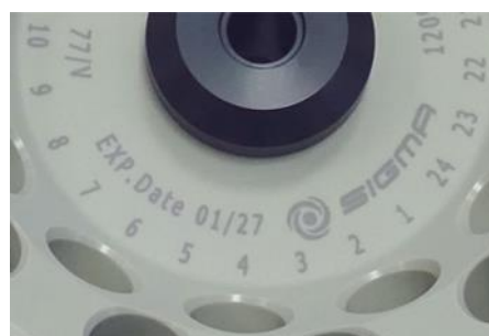
Fig. 5: Different service life – engraving on the bucket/rotor
