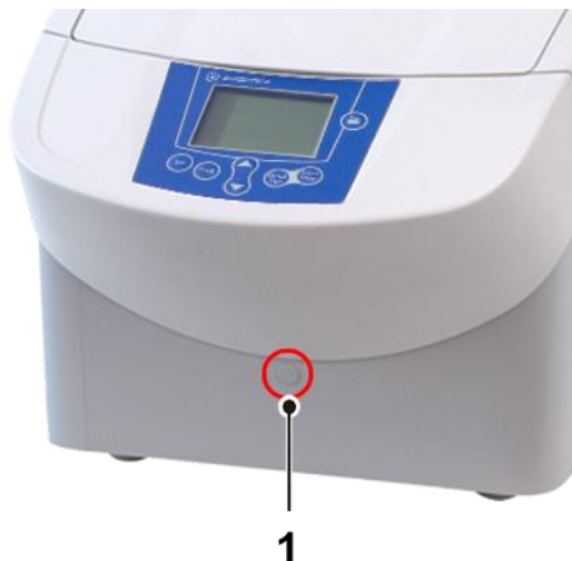
Fig. 8: Position of the opening for the emergency lid release
