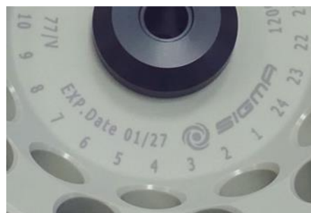
Fig. 4: Different service life – engraving on the bucket/rotor
