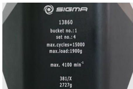
Fig. 4: Different service life – engraving on the bucket/rotor
