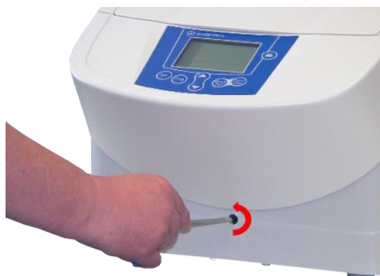
Fig. 9: Manual release of the lid lock
