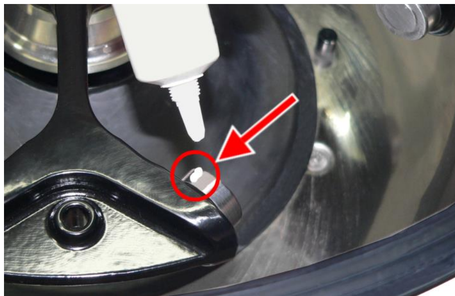
Fig. 33: Sufficient quantity of grease for one bolt
