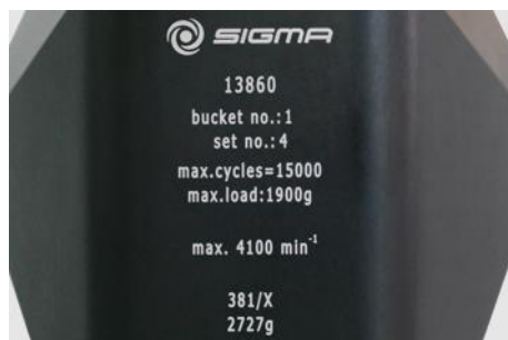
Fig. 5: Different service life – engraving on the bucket/rotor
