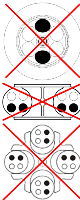
Fig. 19: Permissible and impermissible loading of an angle rotor and a swing-out rotor (example illustrations)
