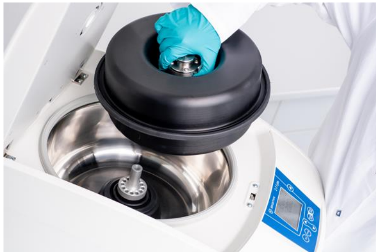
Fig. 15: Installing the cytology rotor
