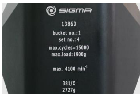
Fig. 5: Different service life – engraving on the bucket/rotor
