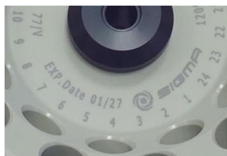
Fig. 5: Different service life – engraving on the bucket/rotor
