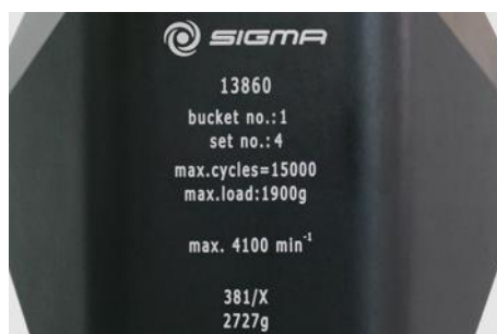
Fig. 7: Different service life – engraving on the bucket/rotor
