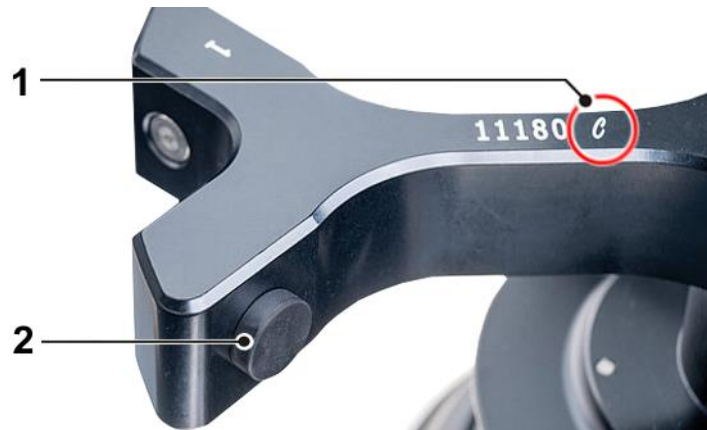
Fig. 9: Marking of a rotor with "Comfort" coating (example)
