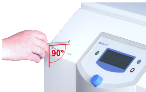
Fig. 39: The emergency lid release key must be inserted horizontally (example illustration)
