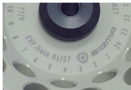
Fig. 7: Different service life – engraving on the bucket/rotor
