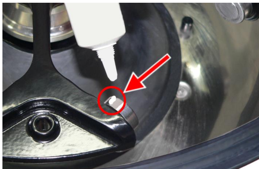
Fig. 40: Sufficient quantity of grease for one bolt
