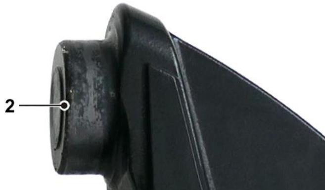
Fig. 10: Load-bearing bolt with traces of use – no greasing required
