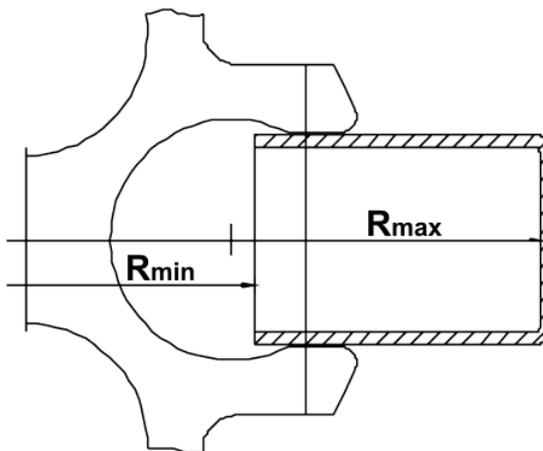
Fig. 48: Minimum and maximum radius of a swing-out rotor
