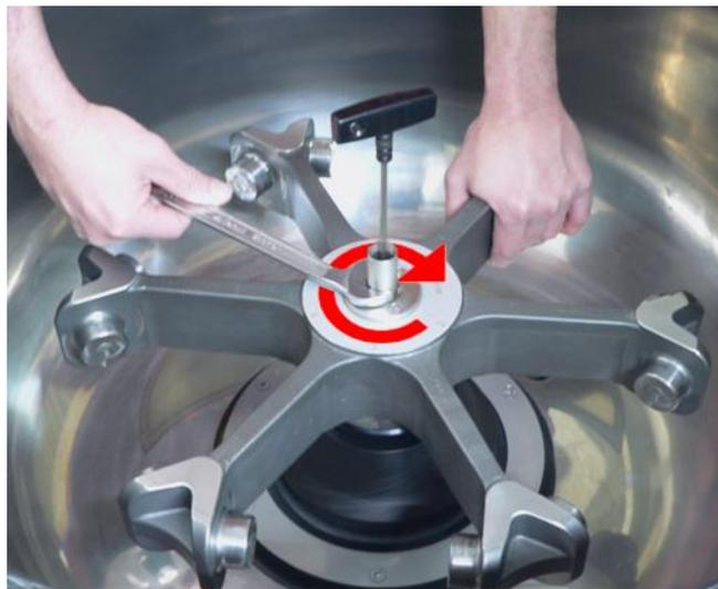
Fig. 15: Fastening of the rotor (example)
