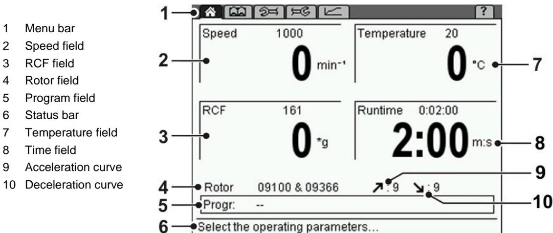
Fig. 24: Display of the Spincontrol S control system
