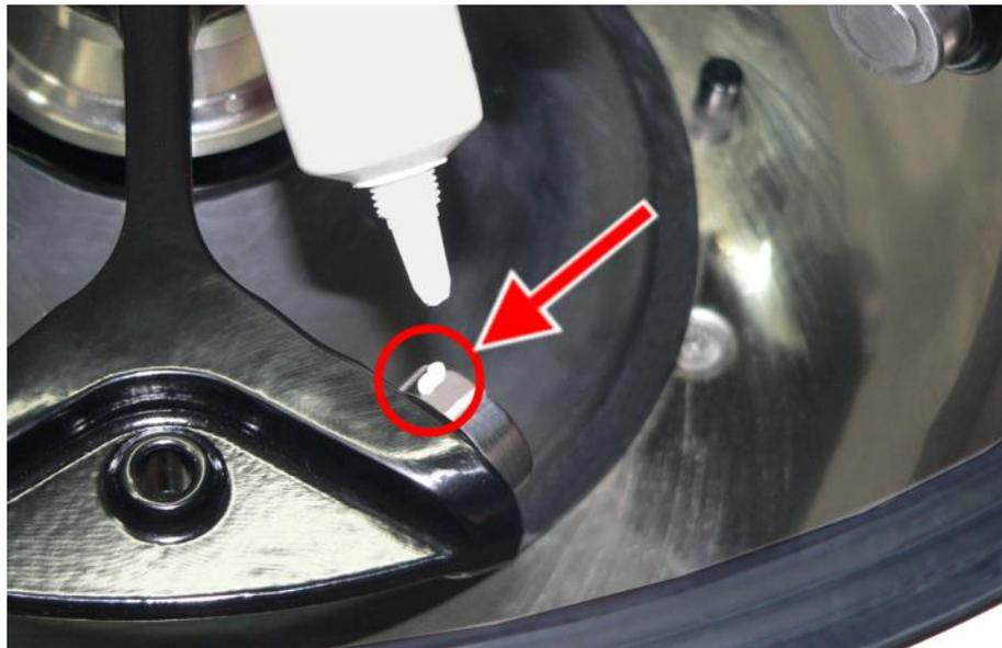
*Fig. 46: Sufficient quantity of grease for one bolt*
