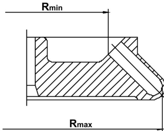
Fig. 47: Minimum and maximum radius of an angle rotor
