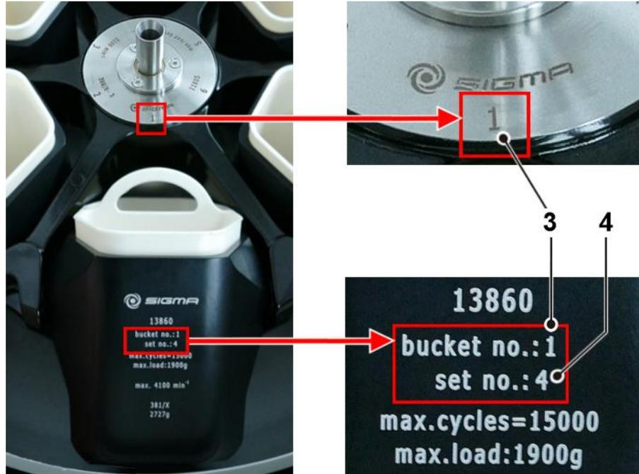
Fig. 10: The bucket number and set number on the bucket and the bucket number on the rotor
