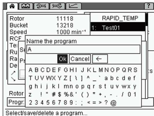
Fig. 39: Assignment of a program name prior to saving the program
