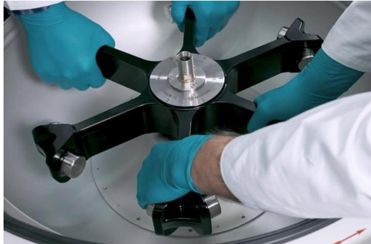
Fig. 16: Correct method for lifting the rotor 11805
