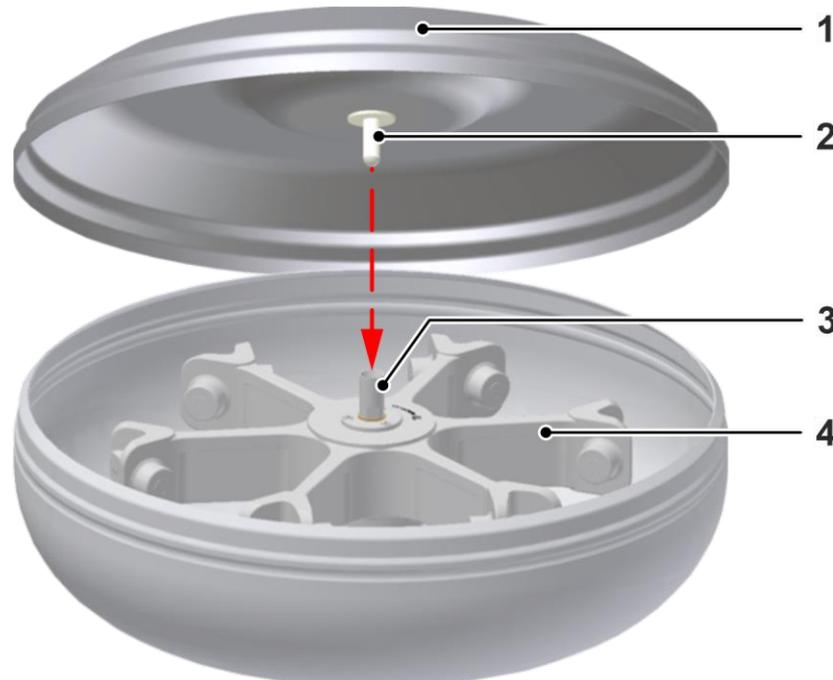
Fig. 17: Lowering the cover onto the windshield
