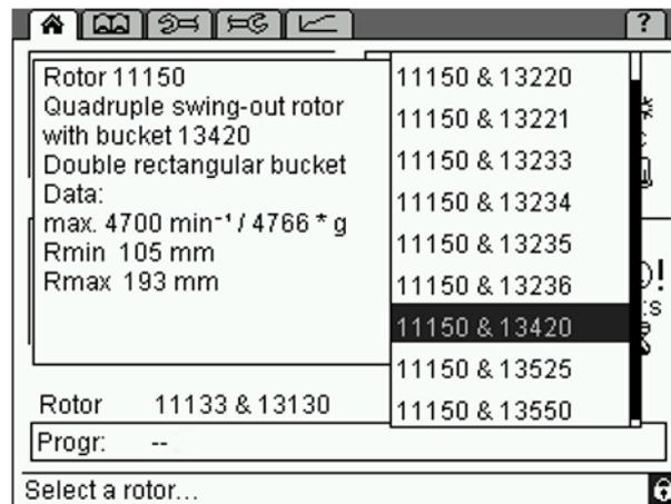
Fig. 26: Rotor selection list, here with potential rotor-bucket combinations and additional information
