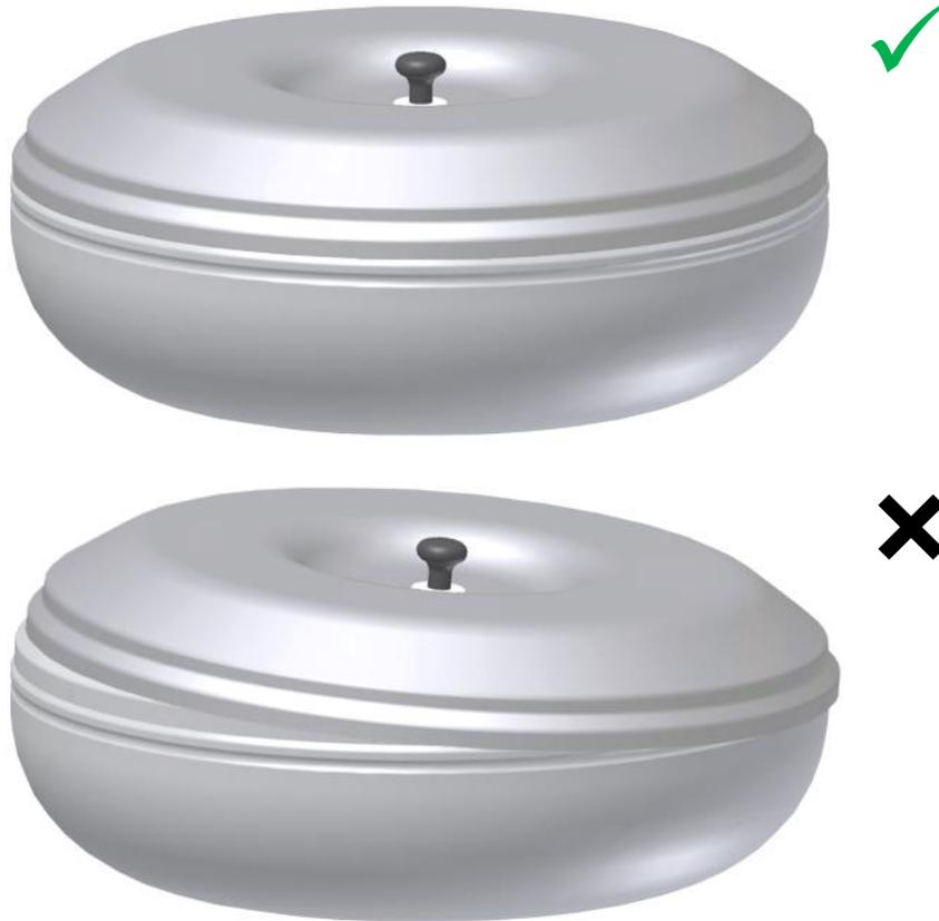
Fig. 18: Checking the cover for correct fit
