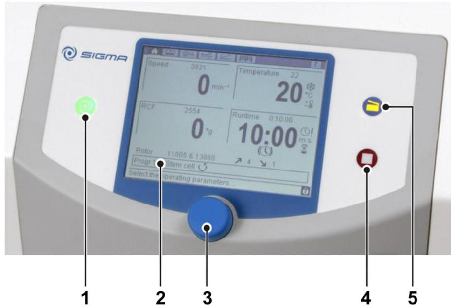
Fig. 23: User interface of the Spincontrol S control system
