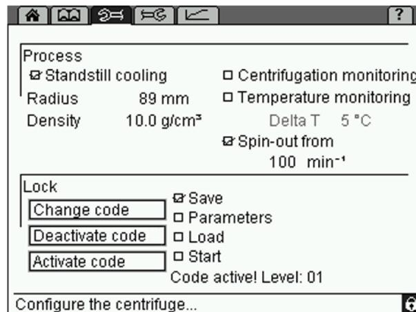
Fig. 33: "Parameters" menu with an active lock (level 01)
