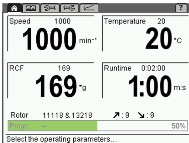
Fig. 29: Progress indicator during a centrifugation run
