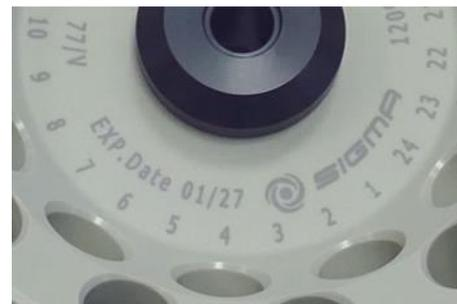
Fig. 8: Different service life – engraving on the bucket/rotor
