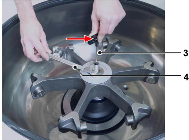
Fig. 14: "Two-finger-principle" for holding the hexagon key (example)
