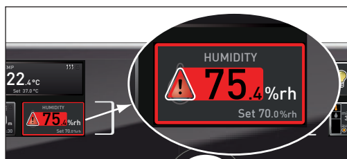
Fig. 22 Humidity monitoring triggered
