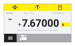
> You can read the measured value as soon as the weight value stops changing and the unit is displayed.
