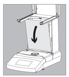
If required, remove the rear panel for cleaning.
