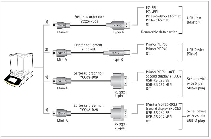
The following connections to peripheral devices are possible:
