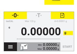
The Checkweighing application appears. The set thresholds are displayed under Min and Max.
