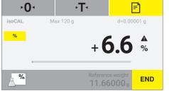
▷ The balance shows the percentage of the sample based on the reference sample.
