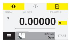
The Counting application appears. The piece count of the reference sample is displayed under Reference.
