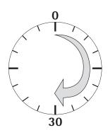
To ensure accurate results are delivered, the scale must warm up for at least 30 minutes after initial connection to the power supply. Only then will the device have reached the required operating temperature.
