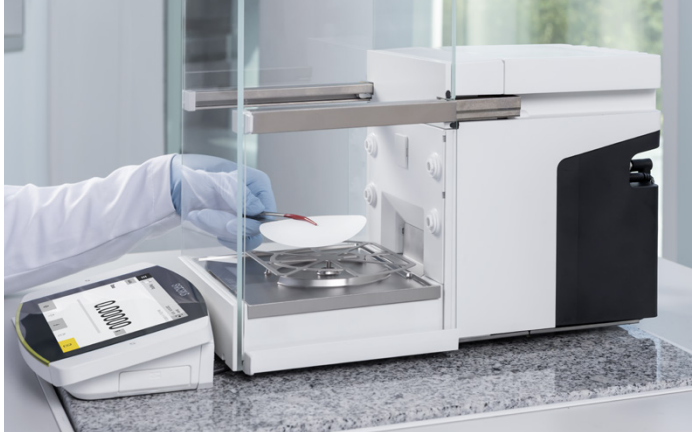
Figure 6: Weighing of charged samples is no problem thanks to the built-in ionizer in the Cubis® II Ultra-High Resolution Balances.
